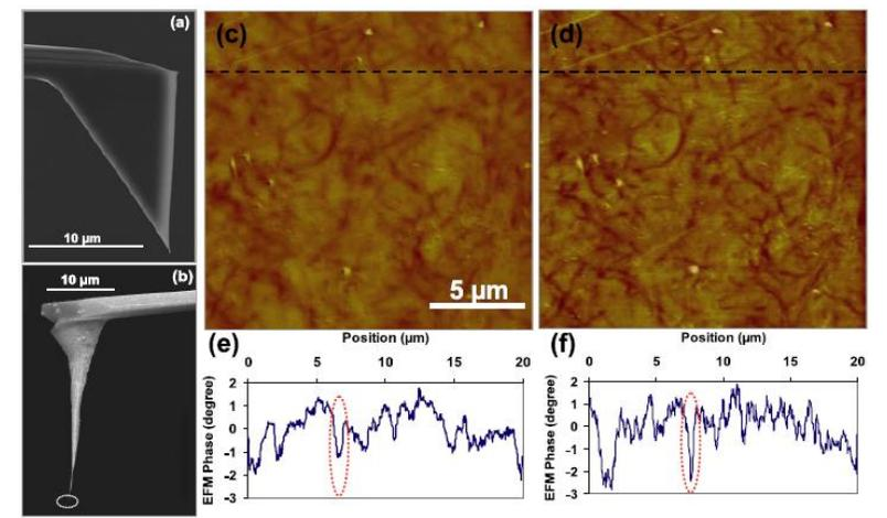
**Figure 3.** Enhanced EFM subsurface imaging of 0.5% SWCNT (LA)-polyimide nanocomposite film using an HAR-NP probe and compare with standard AFM probes. *Nanotechnology* 21 (2010) 225702
