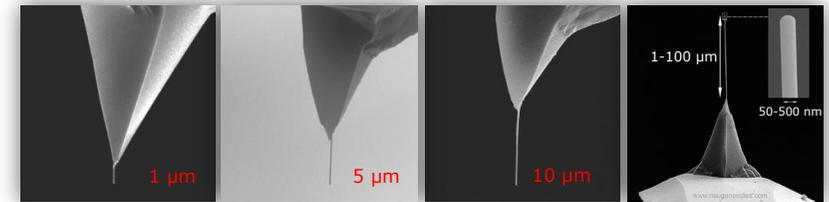
*Figure 1 SEM image of High Aspect Ratio Needle-Probes*
