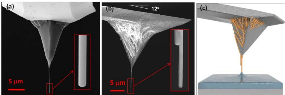
*Figure 1 SEM image of Needle-Probes (a) with single nanoneedle and (b) double nanoneedle) which show a simple geometry of the nanoneedles, (c) schematic of a double-nanoneedle being dipped in a liquid surface.*
